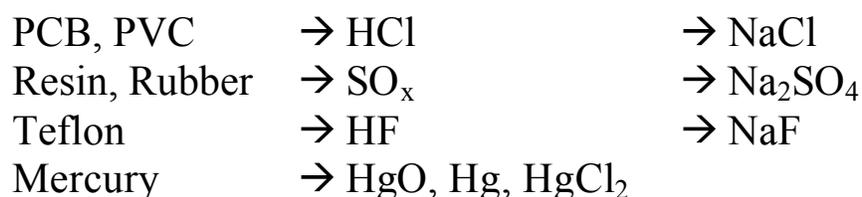
Fig. 3. Scrubber Chemistry Neutralizes Acid Gases by Forming Low-Volume Salts
