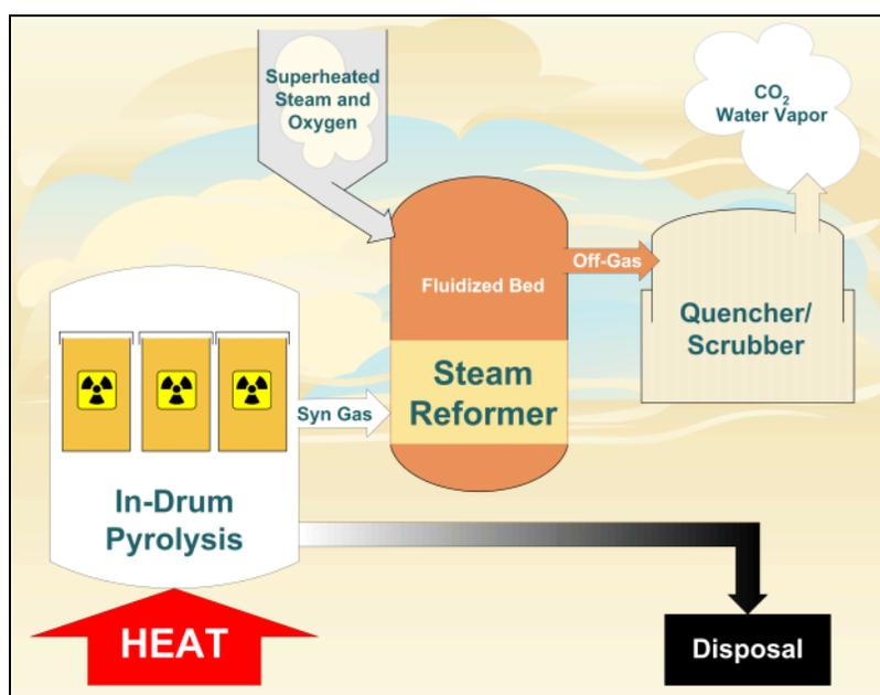
Fig. 1. Conceptual representation of the THOR<sup>SM</sup> pyrolysis and steam reforming systems
