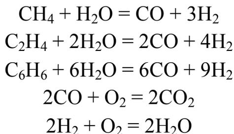
Fig. 2. Conversion of Volatized Hydrocarbons into Carbon Dioxide and Water Vapor
