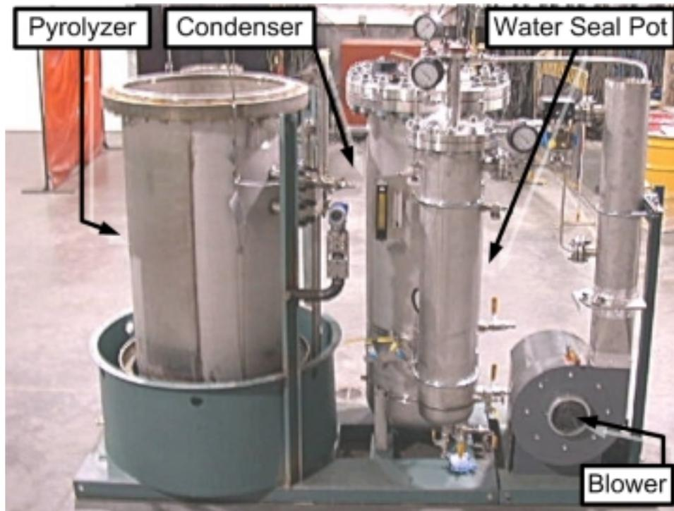
**Fig. 1. The THOR<sup>SM</sup> Drum Autoclave Test System Shown Without Insulation Blankets**
