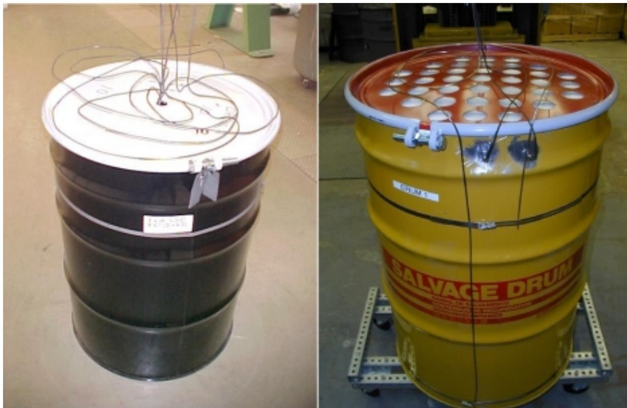
**Figure 2. Assembled 55-gal. drum (left) and assembled 85-gal. overpack containing a 55-gal. drum (right)**
