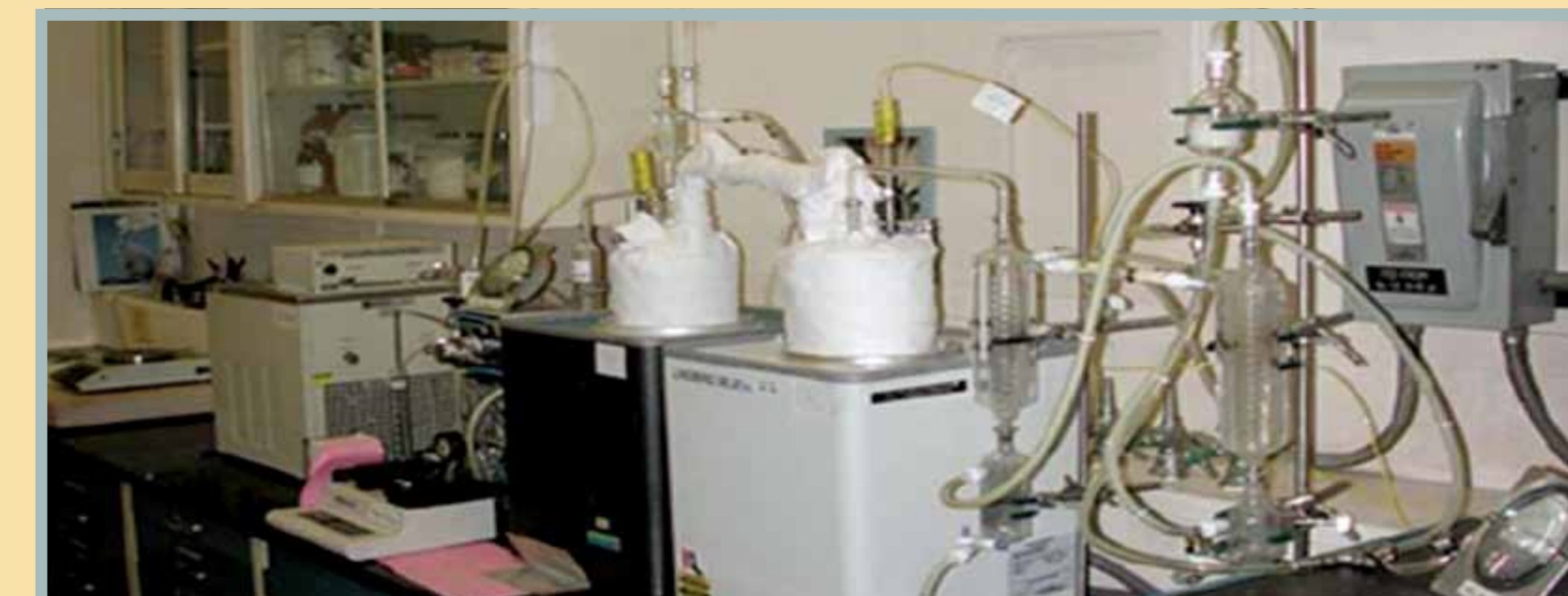
Bench Scale Reformer (BSR) at SRNL is being used to demonstrate on a laboratory scale the processing of a radioactive simulated LAW or LAW Recycle
