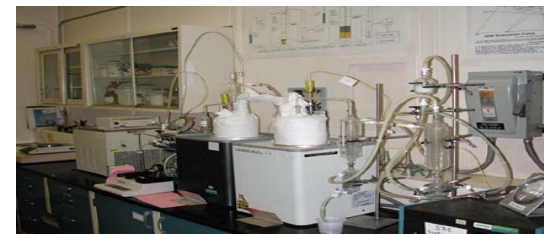
Bench Scale Reformer (BSR) at SRNL is being used to demonstrate on a laboratory scale the processing of radioactive simulated LAW or LAW Recycle.
